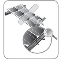
Do Not reconnect or repair junction box cable. It may occur spark or electric shock.
