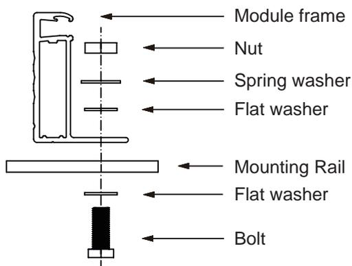
\* Mounting Rails Material : Aluminum, Stainless steel, etc.
