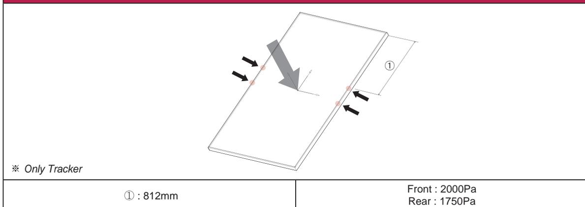
Note) When installed Fig.7, follow the tracker manufacturer's recommended applied torque and materials to fasten the modules.
