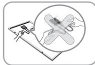
If the installing modules on curved surface, (e. g. arch type), as shown in the below picture, do not forcefully modify the module in the installation when connecting it with the structure. Only install the module in the place where the structure for the panels has been properly set up. An improper structure may cause deformation of the panels. Panels may also be damaged by unapproved installation methods such as the use of a crane.
