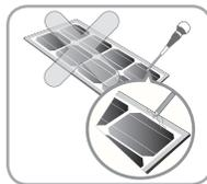
Do not artificially concentrate sunlight on the solar module surface. Failure to comply may result in product damage or failure.
