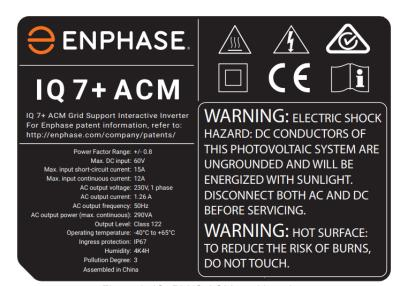
Figure 2: IQ7PLUS ACM marking plate
