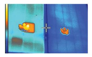
Conventional Module JinkoMX-Enabled Module Eliminate hot spots with JinkoMX enabled modules.
